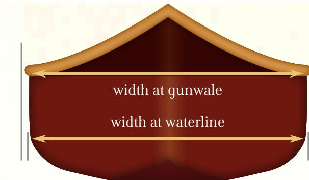
Measured at the widest point of the canoe and largely impacts stability and speed. The most common reference is width at the gunwales but an often more telling dimension is width at the waterline as this will determine the amount of effort required to move the boat through the water.
