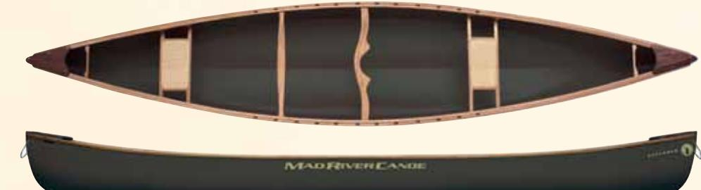
Crafted with an Explorer hull (olive drab in and out), this timeless canoe is fashioned with classic cane seats along with dark stained slotted ash gunwales, thwart and yoke.
