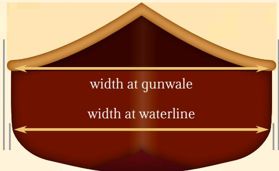
Measured at the widest point of the canoe and largely impacts stability and speed. The most common reference is width at the gunwales but an often more telling dimension is width at the waterline as this will determine the amount of effort required to move the boat through the water.
