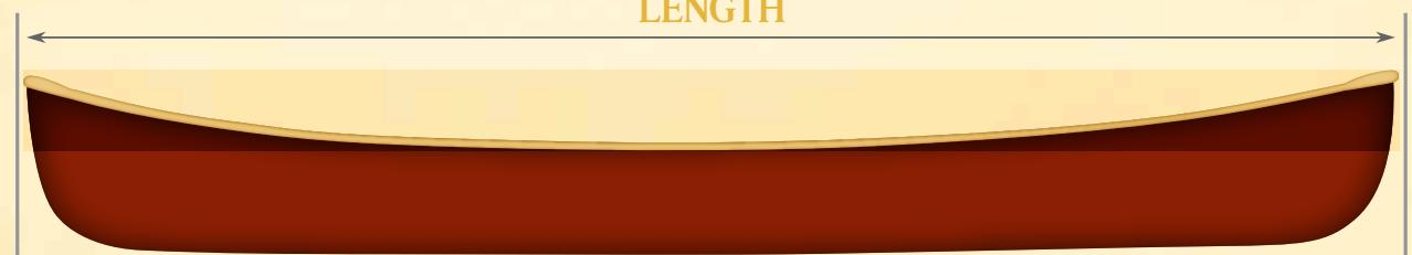
Measured stem to stem and is the most straightforward of all the aspects of canoe design. In terms of versatility, canoes in and around 16' are preferred. Large enough to be paddled tandem with a load or soloed on occasion and fast enough for touring yet nimble enough to work their way down a twisty stream. Canoes with emphasis on cruising speed tend to be longer while whitewater canoes shorter with a premium on maneuverability.
